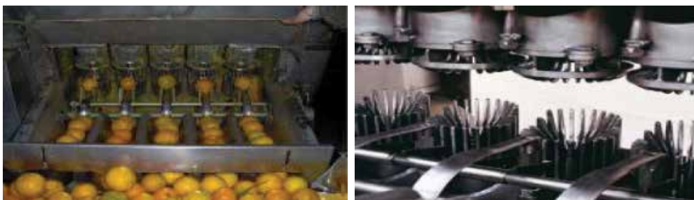
Figure 14 – Extractor Cups and Kinnow Feeding into Extraction
